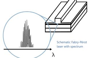
Any **custom wavelength** is possible: You tell us what you need! With our outstanding technology we design any wavelength **between 1950 nm and 2350 nm** with an accuracy of +/- 20 nm. Other wavelengths are available on request.
