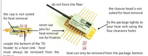
bottom In the shown TO5 case, the laser-chip is soldered on top of a heat spreader, which is mounted to the TEC. The bottom of the TEC is attached to the TO5 base plate of the header. Because of thermal radiation and air currents, it is advisable to enclose the laser mount in some sort of con-
